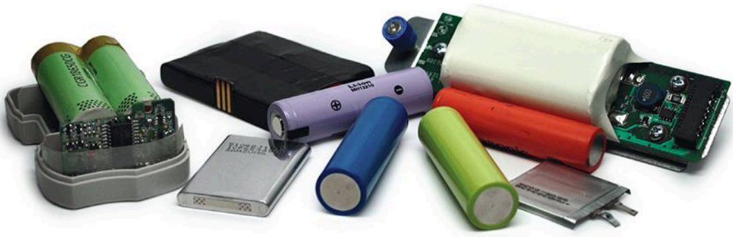
1. Shown are examples of Li-ion cells incorporated into battery packs with electronics and either hard-plastic enclosures or shrink-wrapping.
