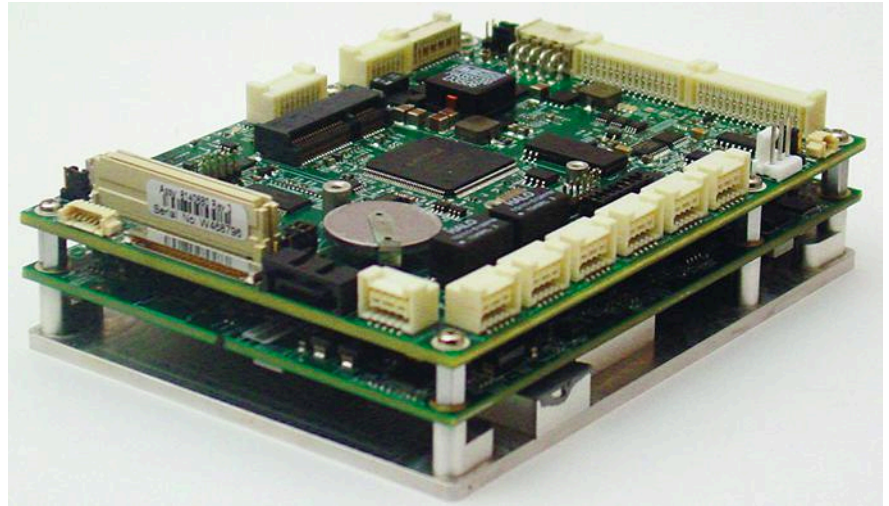
2. Diamond Systems' Vega is an EMX form factor that hosts a COM Express board to provide processing options.
