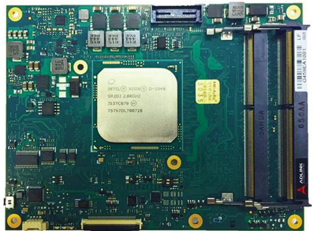
1. ADLINK's Express-BD7 is a Type 7 COM Express board that exposes a 10 Gbit/s Ethernet interface.
