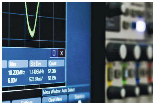
6. Shown is standard deviation of a signal after 58,000 measurements on an InfiniVision 6000 X-Series oscilloscope.
