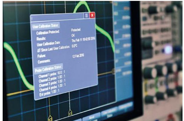
4. User calibration status is provided on a Keysight InfiniiVision 4000 X-Series oscilloscope.
